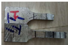
Figure 3. Test specimen of tensile after fracture
