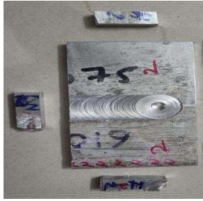
Figure 5. Test specimen of impact after fracture
