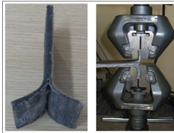
Fig 5: Optical image of delamination test sample and test setup.
