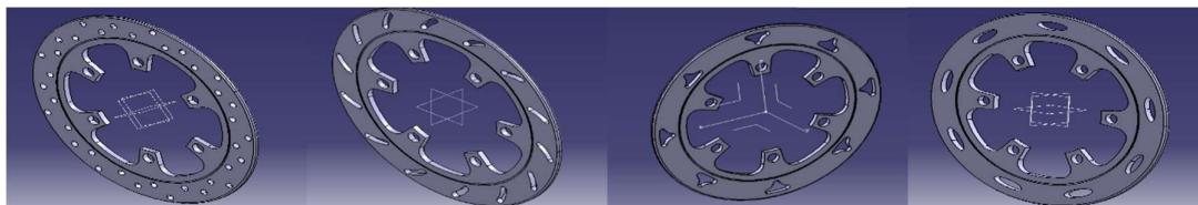
Figure. 5. 3d drilled disc Figure. 6. 3d slotted disc Figure. 7. 3d clouded disc Figure. 8. 3d elliptical disc
