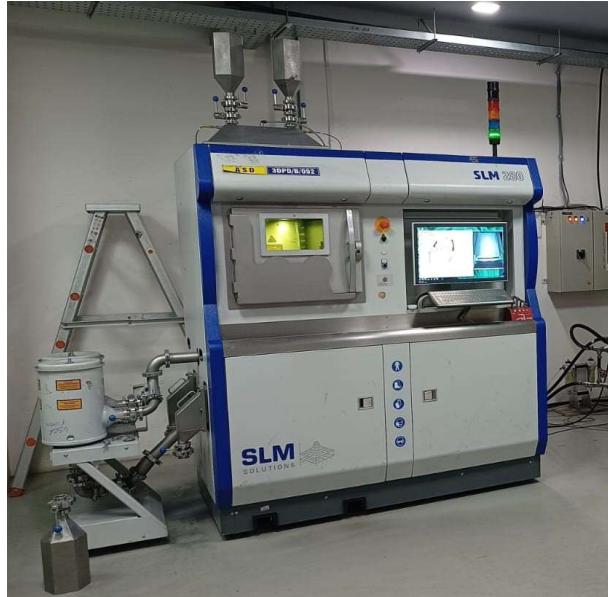
Fig. 2 SLM 280 Setup (Courtesy- 3D Product Development Pvt. Ltd.)
