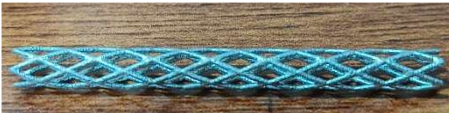
Fig. 3 3D Printed SS316L powder stent with SLM process
