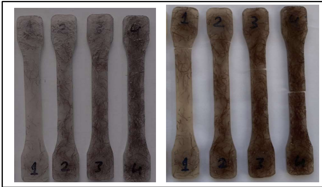
Figure 3: Tensile specimens pre and post testing.
