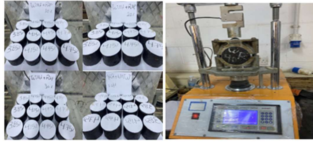
Figure 5. Marshall test WMA sample in machine
