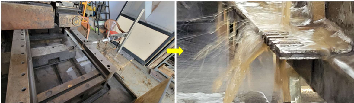
Fig.3 Powder mixed electric discharge machining (PMEDM)
