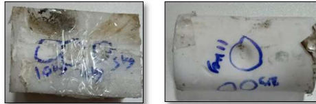
Figure 5. Nature of Specimens after Impact
