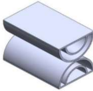
Figure 2. Double Half Cylinder Model of Energy Absorption
