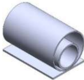
Fig.1. Double Cylinder Energy Absorber
