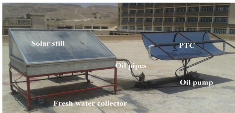
Figure 7: Single slope still in an experimental configuration with PTC (Fathy et al., 2018)
