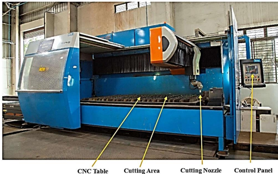
Fig. 1. Experimental set up of laser cutting process
