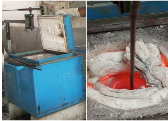
Figure 1: The electrical resistance furnace with stirring of Aluminum 2285 – 4wt.% Si 3 N 4 – 6wt.% Mullite Hybrid MMC molten metal
