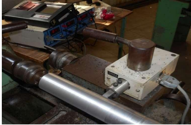
Figure 3: Machining of Al2285 – 4 wt.% Si 3 N 4 - 6% wt.% Mullite Hybrid MMC specimen
