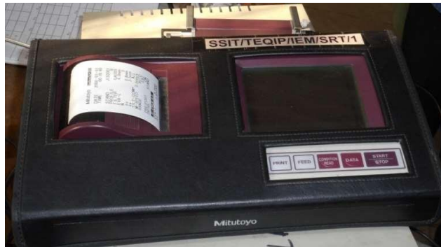
Figure 4: Surface roughness measuring instrument
