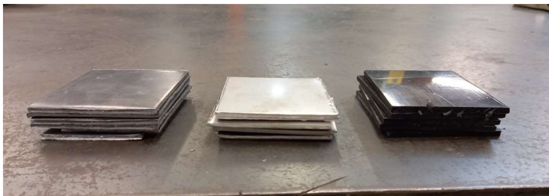
Figure 2: Samples after being cut to desired shapes, mild steel, stainless steel, and HDPE (left to right).
